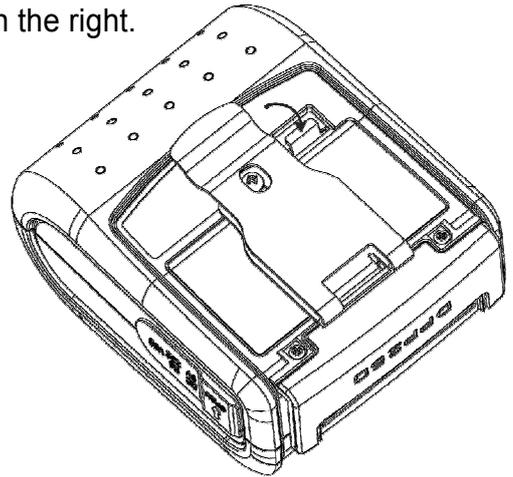
2. Lift the battery cover as shown in the figure on the right.
