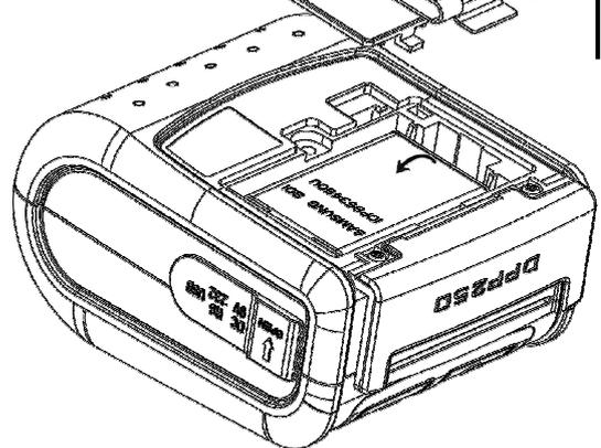
4. Detach the battery as shown in the figure on the right.
