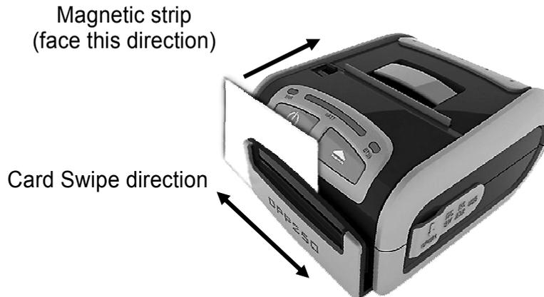
The reader's magnetic head faces towards the front of the printer. When placing the card into the reader, the magnetic strip must be facing as show in the figure above. Keep the bottom edge of the card flat on the inner base of the reader to ensure that the magnetic strip passes over the read head evenly.
